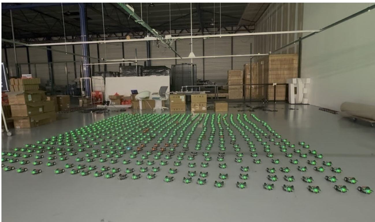
Figure 1: The OpenSwarm testbed of 725 DotBots.
