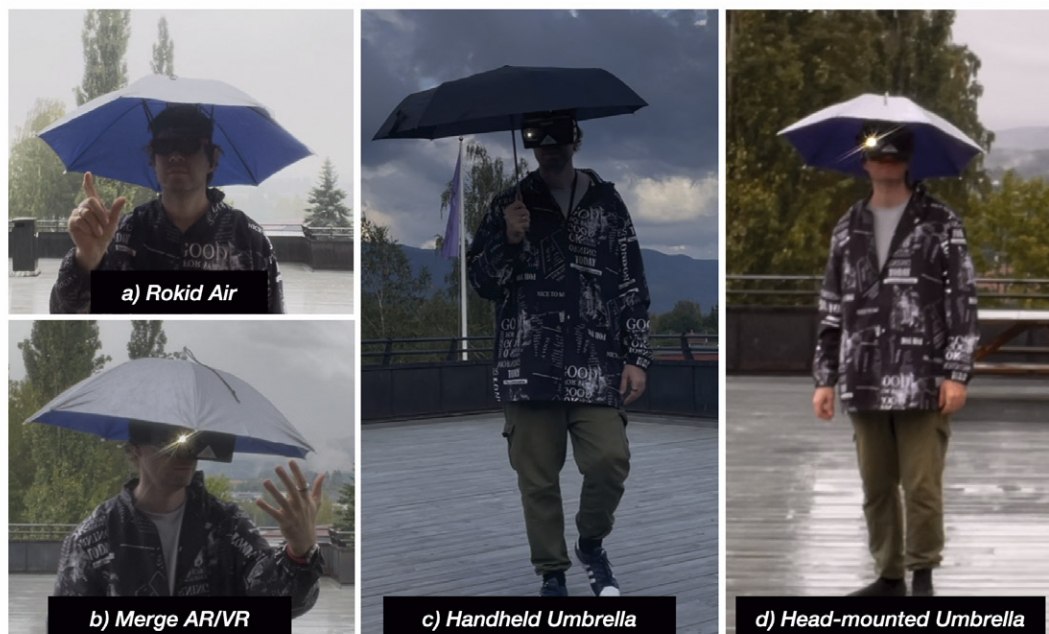
Figure 1: Outdoor pilot with AR. (a) Rokid Air used in rain with a head-mounted umbrella. (b) Merge AR/VR used in rain with a head-mounted umbrella. (c) Testing with a traditional handheld umbrella. (d) Testing with a head-mounted umbrella in the rain.
