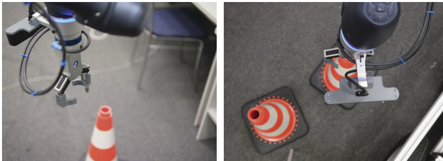
Figure 3: The robot arm, equipped with a stereo camera, scans the robot platform's environment and positions itself to collect the cone.
