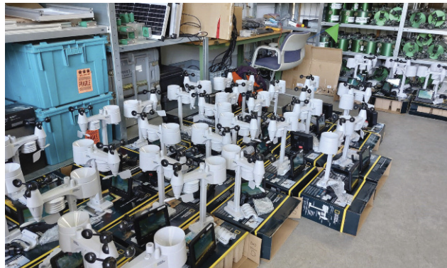
Figure 1: National Geographic Weatherstations being assembled and tested before sending to the pilot cities for use by citizen scientists to collect local climate data.
