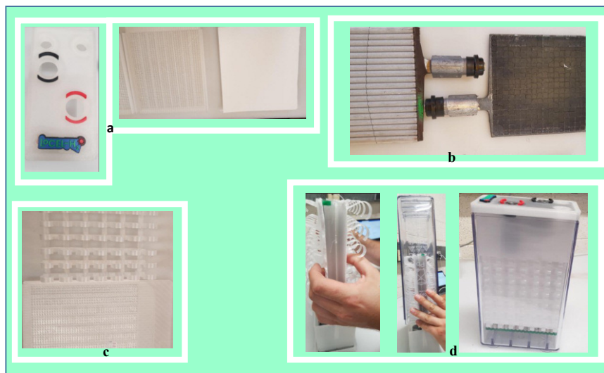
Figure 1: a) A new 3D-printed lid and separator frame with gas flow channels. b) Plates provided by Hoppecke and soldered to terminal blocks. c) An H&V separator was located within the new separator frame and H&V AGM and printed spring clips were used to provide pressure to the plates. d) Manufacture is straightforward – connect the terminals, assemble and slide the battery box on. Bubbles of hydrogen ( H_2 ) and oxygen ( O_2 ) appear at the output ports under electrolysis.
