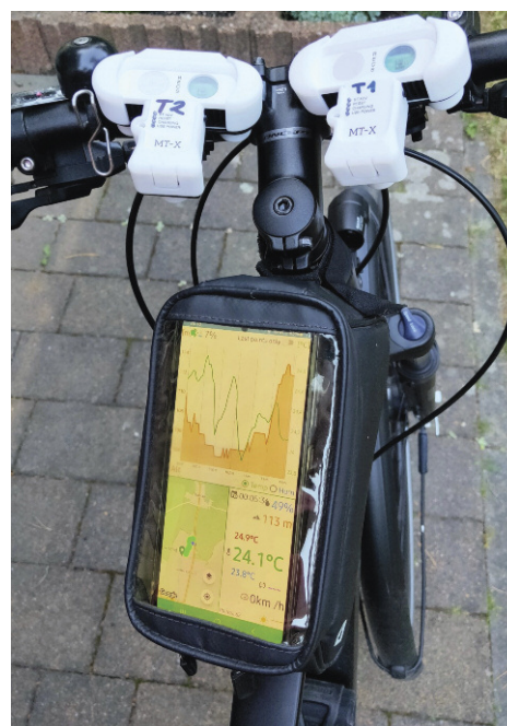
Figure 2: MeteoTracker mobile climate sensors for use by citizen scientists on their bicycles. The data is visible to citizens and researchers via a dashboard, instantly visualising the diverse climate conditions of a city in an accessible way.
