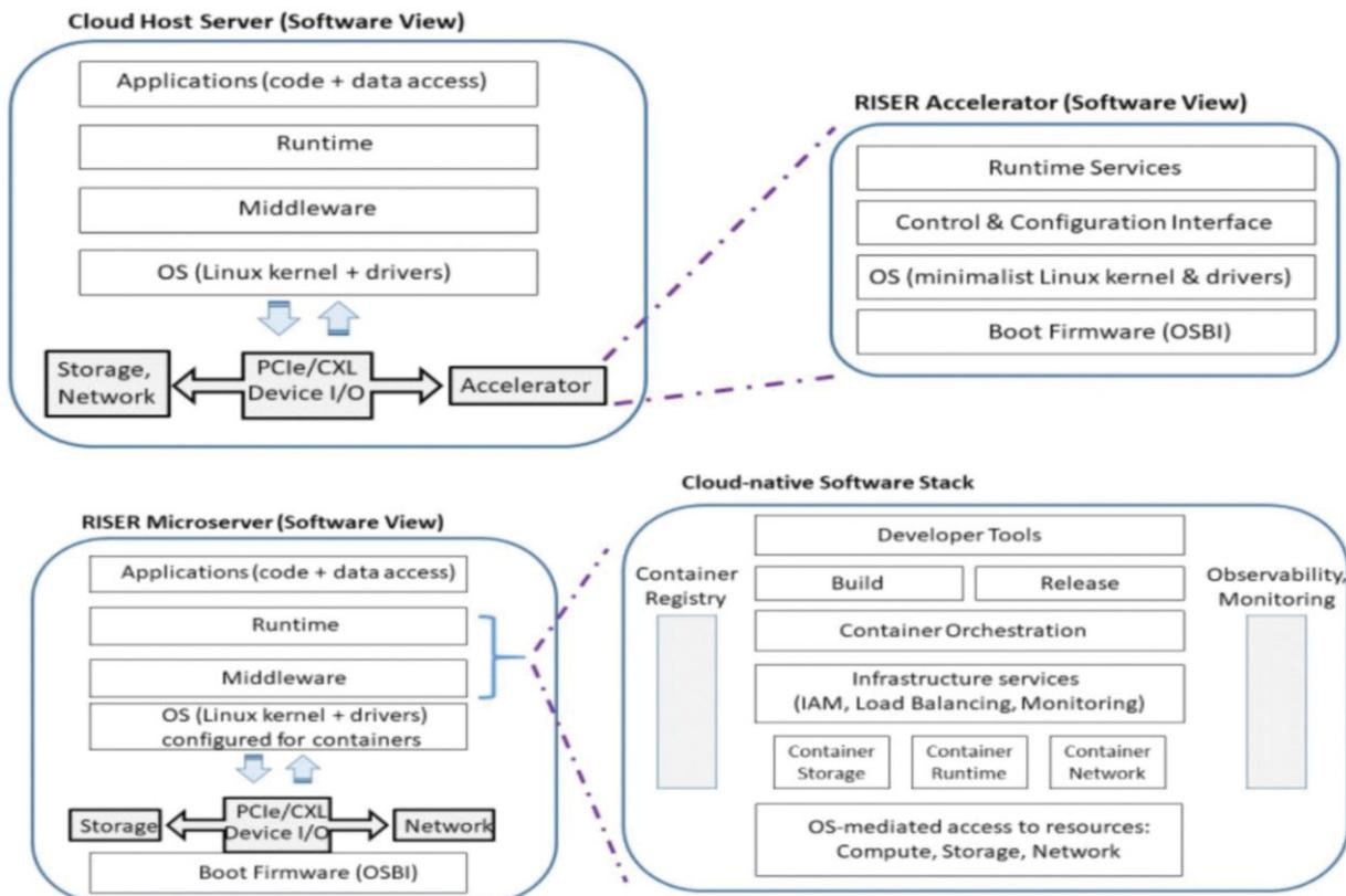
Figure 2: System software for the two RISER platforms: accelerator interacting with host, and microserver with cloud software stack
