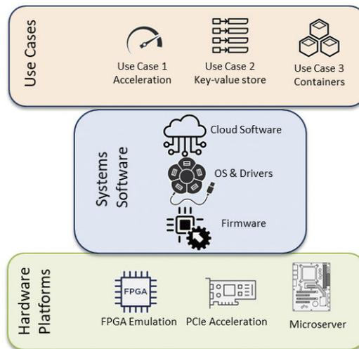
Figure 1: RISER Architecture logical layers.
