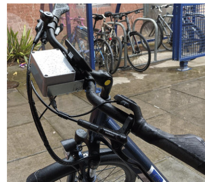
Figure 1: The E-bike Telematics System: (left) the devices fitted to a host e-bike during a lab trail. The lid of the waterproof enclosure has been removed to expose the internal electronics; and (right) the device after it has been fitted to an e-bike as part of the two-year-long REPLICATE technology deployment.
