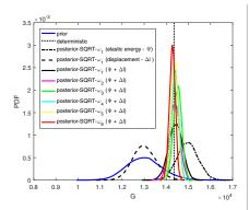
Figure 2: Comparison of prior and posterior pdf functions for shear modulus bulk modulus performed on uniaxial compression test obtained by SQRT Kalman filter (six realisations on micro-scale  $- w_6$ ).
