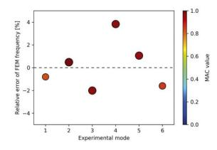
Figure 1: Results obtained by the calibrated finite element model in comparison with the experimental data: relative error in frequency and modal assurance criterion (MAC) value.
