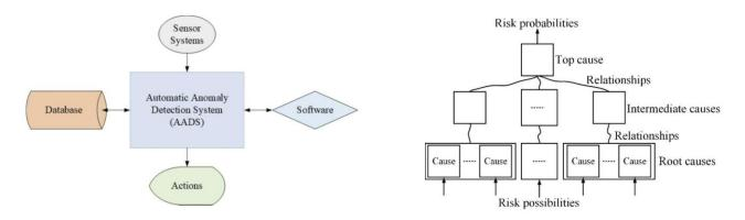
Figure 1: AADS model. Left (a) General framework of AADS for fully autonomous ships, right (b) Form of Risk Structures for AADS
