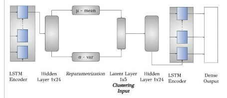
Figure 1: Variational recurrent neural network layer stack.
