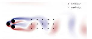
Figure 2: Vorticity field for the unforced natural flow at Reynolds
