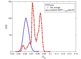
Figure 3: Updates for softening parameter  $G_{f,c}$  (fracture energy) obtained by SQRT Kalman filter with three measurements taken from uniaxial compression test for 20 different realisations –  $w_{2fr}$
