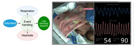
Figure 1: A high-level functional block diagram of our real-time, continuous monitoring system (left), and a typical display view showing the extracted waveforms and rate estimations along with object detection overlay (right).
