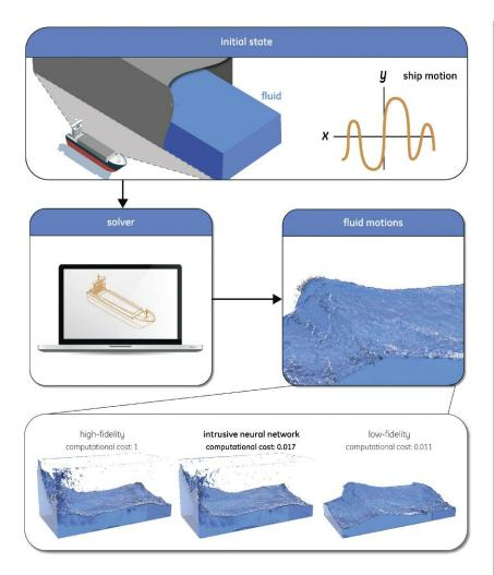
Figure 1: Intrusive neural networks can be used, for instance, to predict sloshing in a very effective and efficient way, making it possible to use it as a predictive tool for decision making. Our new method to solve Navier-Stokes equations for this and other applications in engineering is about 100 times faster than before, whilst maintaining almost the same accuracy. Picture: CWI.
