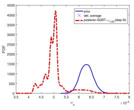
Figure 4: Updates for softening parameter  $s_u$  (limit stress) obtained by SQRT Kalman filter with three measurements taken from uniaxial compression test for 20 different realisations –  $w_{20}$
