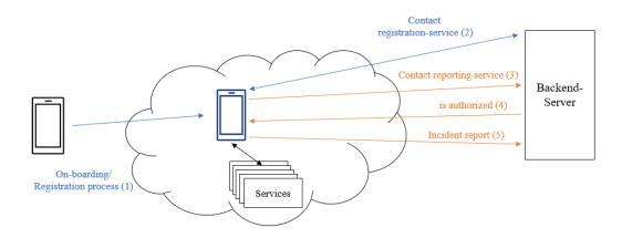
framework Arrowhead, which provides many security functions by design. First, smartphones can be onboarded in the Arrowhead framework, as shown in Figure 1. They form part of the Arrowhead local cloud, authorised by certificates, and can share information in a trustworthy way, e.g., reporting incidents in the context of "Civis 4.0 Patria".
