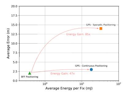
Figure 1: Average error vs average energy required per position fix for the positioning technologies discussed in this article. The proposed BFF positioning system has an accuracy comparable to low-power GPS implementations, while achieving energy efficiency gains exceeding 47× per position fix.
