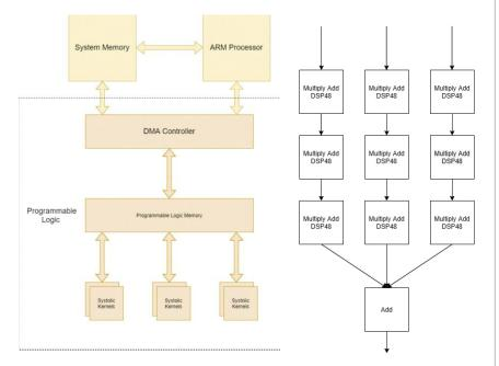
Figure 2: System Level architecture of the proposed solution.
