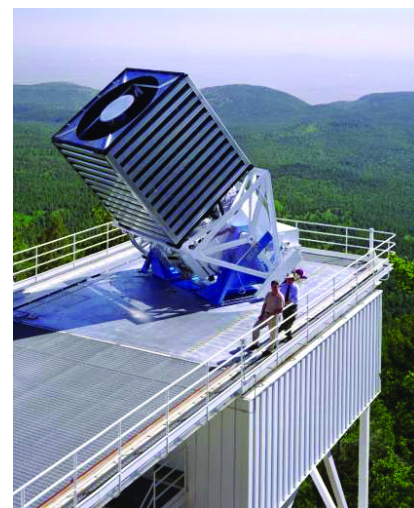
Figure 2: The Sloan Telescope, a 2.5-meter telescope at Apache Point Observatory, did all SDSS imaging and spectroscopy. (Picture: The Sloan Digital Sky Survey.)
