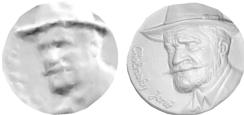
Figure 2: left: surface measured by laser scanner; right: textured model.
