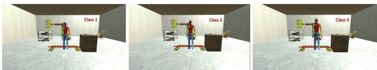
Figure 3: Examples of the simulator in different configurations (height of the operator), for ergonomic analysis in a safe virtual environment.
