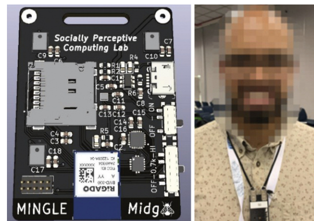
Figure 1: The MINGLE Midge Smart ID badge (left). Demonstration of how it is worn with a black lanyard around the neck (right). It contains a 9-degree-of-freedom inertial measurement unit, Bluetooth transmitter and receiver for measuring proximity to other sensors, and the possibility of recording high or low frequency audio for assisting in the training of body-language-based models. The design is open source. More details and access can be found at [1] and [L1].
